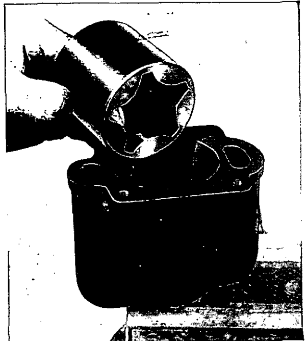
Fig. K.7. Replacing Outer Rotor.
