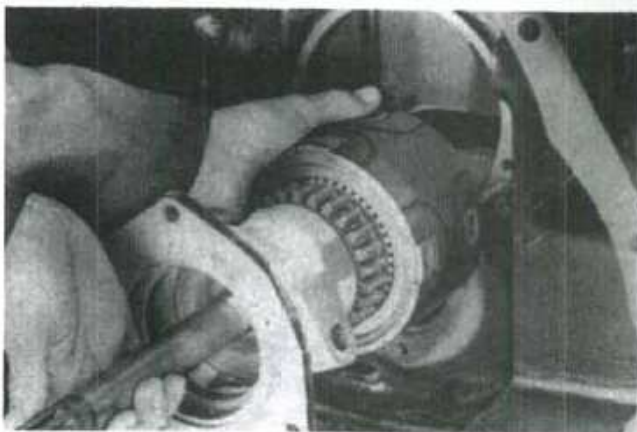
Fig. 106—Remove Forward-Reverse unit from front of speed gearbox.
