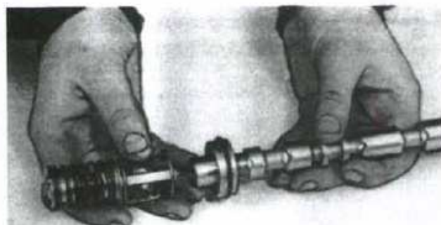
Fig. 173—View of detent assembly removed from valve spool. Do not disassemble detent unit as no parts are available.
