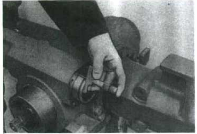
Fig. 43—Using a depth gage, measure distance between axle housing and end of cylinder sleeve. Refer to text.
